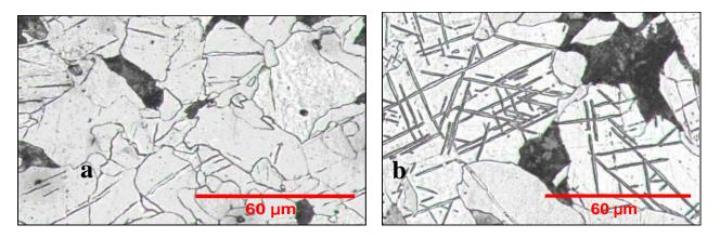
Figure 5. Example of optical micrographs of post impact steel specimens a.) 7 GPa peak stress yielding 3.4% twins, b.) 9 GPa peak stress yielding 4.3% twins.
