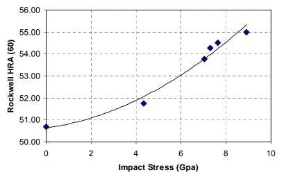
Figure 6. Post-impact macro hardness as a function of impact stress
