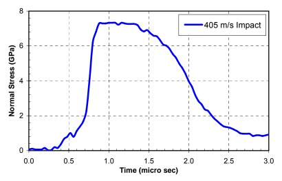
Figure 3. Impact Stress recorded with manganin gauge at the back surface of target disk during a 405 m/s impact
