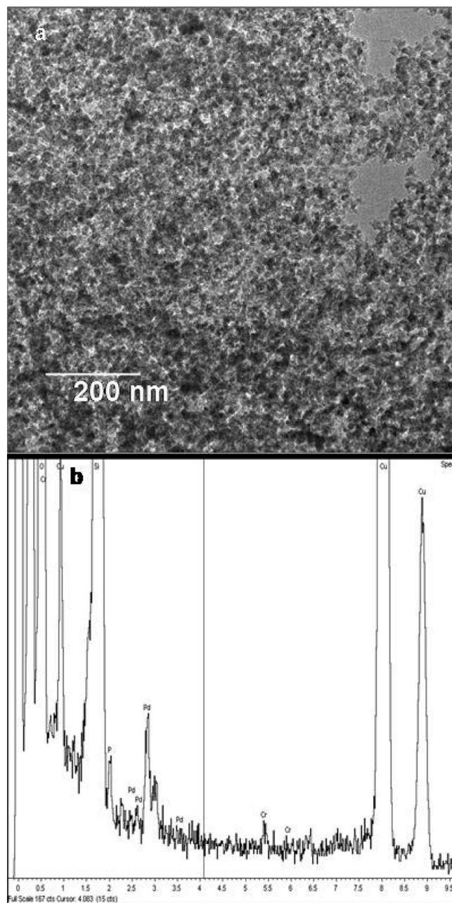
**Figure 5.** Example of TEM image showing APTES functionalized bulk silica with palladium nanoparticles covalently attached to its surface (a) and EDS spectrum which reflects the presence of both Pd and Si (c). The Cu peaks are due to the copper TEM grids.
