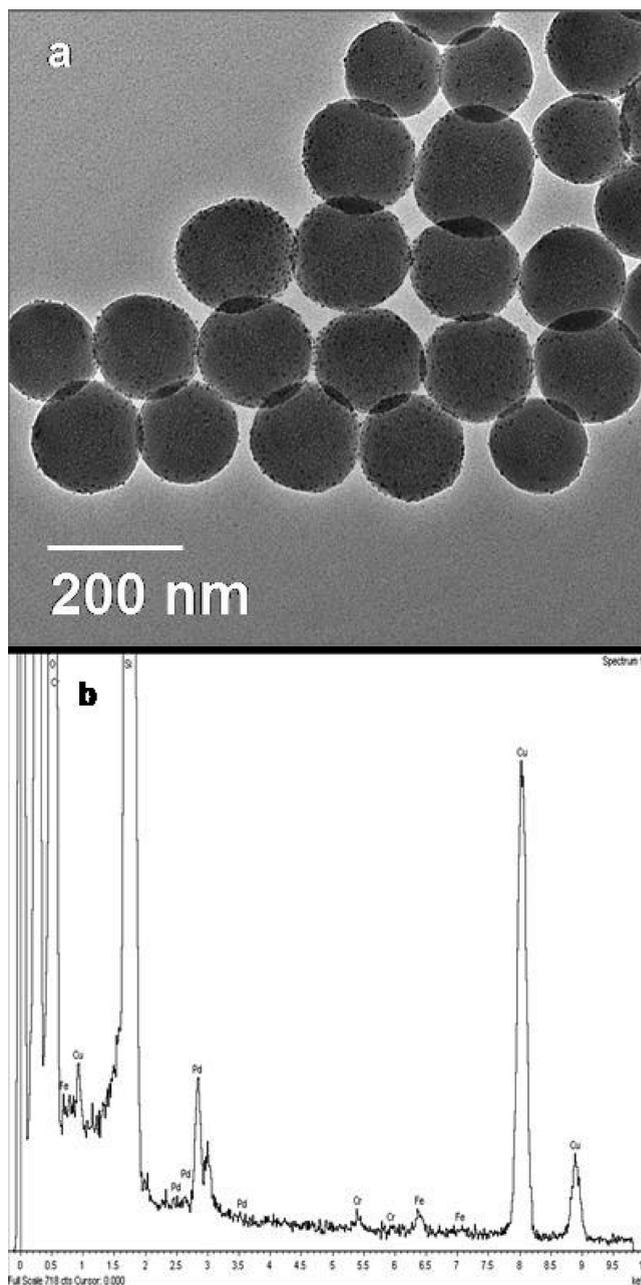
**Figure 3.** A representative TEM image showing the palladium nanoparticles covalently bound to APTES functionalized dried silica colloid suspensions (a) and EDS spectrum which reflects the presence of both Pd and Si (b). The Cu peaks are due to the copper TEM grids.
