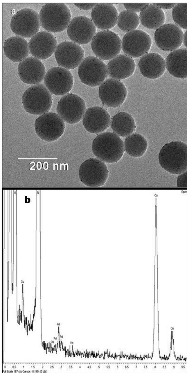
**Figure 2.** Examples of TEM images showing palladium nanoparticles directly adsorbed onto the surface of the silica colloid suspensions (a) and EDS spectrum which reflects the presence of both Pd and Si (b). The Cu peaks are due to Cu TEM grids.
