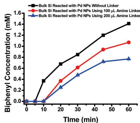
**Figure 12.** Comparisons of the catalytic activity with unfunctionalized bulk dry Si dispersed in doubly deionized water that are air-dried and APTES functionalized bulk dry Si dispersed in doubly deionized water that are air-dried.
