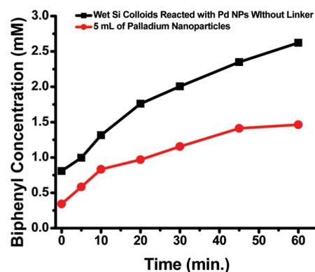
**Figure 9.** Comparisons of the catalytic activity with wet Si colloids reacted with Pd NPs without linker that are air-dried and palladium nanoparticles in colloidal solution.
