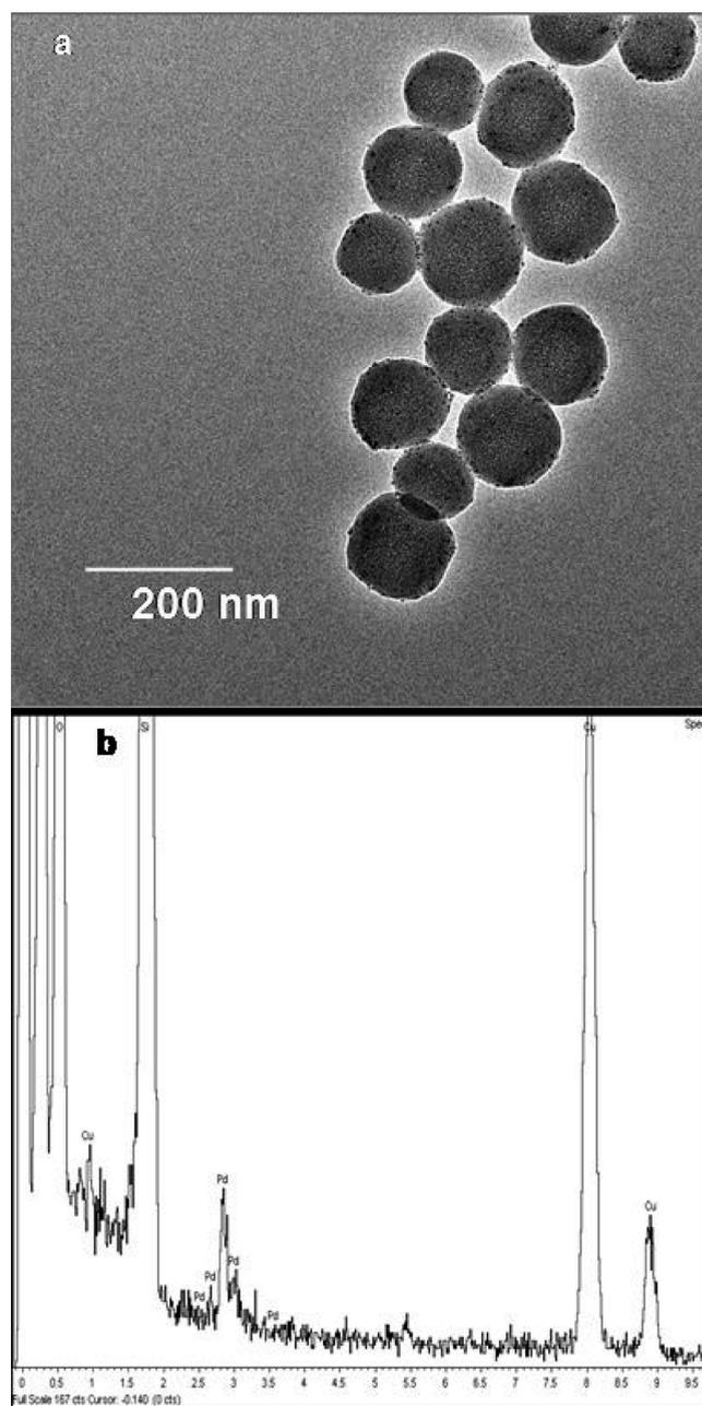
**Figure 1.** Example TEM image showing the palladium nanoparticles covalently bound to amine functionalized silica colloid suspensions (a) and EDS spectrum which reflects the presence of both Pd and Si (b). The Cu peaks are due to the copper TEM grids.
