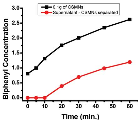
**Figure 13.** Comparison of the catalytic activity of the supernatant solution after refluxing the CSMNs in 3:1 acetonitrile and centrifuging to that of the CSMNs used as catalysts for the Suzuki reaction.
