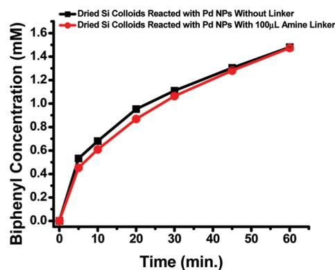
**Figure 11.** Comparisons of the catalytic activity with unfunctionalized dried Si colloids resuspended in doubly deionized water that are air-dried and APTES functionalized dried Si colloids resuspended in doubly deionized water that are air-dried.
