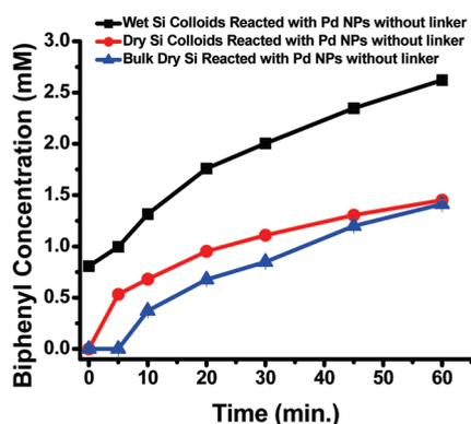
**Figure 8.** Comparisons of the catalytic activity with wet unfunctionalized Si colloids reacted with Pd NPs that are air-dried, dry unfunctionalized Si colloids resuspended in doubly deionized water and reacted with Pd NPs that are air-dried, and unfunctionalized bulk dry Si dispersed in doubly deionized water and reacted with Pd NPs that are air-dried.
