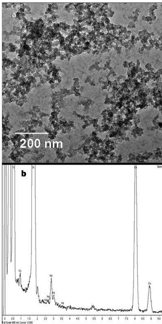
**Figure 6.** Example of TEM image showing unfunctionalized bulk silica with palladium nanoparticles adsorbed to its surface (a) and EDS spectrum which reflects the presence of both Pd and Si (b). The Cu peaks that appear are due to copper TEM grids.
