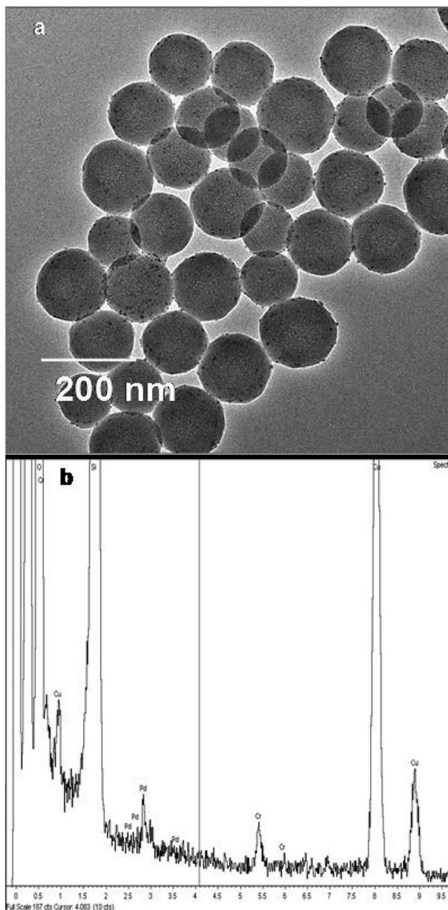
**Figure 4.** A representative TEM image showing the palladium nanoparticles adsorbed onto the unfunctionalized dried silica colloid suspensions (a) and EDS spectrum which reflects the presence of both Pd and Si (b). The Cu peaks are due to the copper TEM grids.
