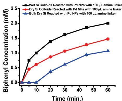
**Figure 7.** Comparisons of the catalytic activity with wet APTES functionalized Si colloids reacted with Pd nanoparticles that are air-dried, dry APTES functionalized Si colloids resuspended in doubly deionized water and reacted with Pd nanoparticles that are air-dried, and bulk dry APTES functionalized Si dispersed in doubly deionized water and reacted with Pd nanoparticles that are air-dried.
