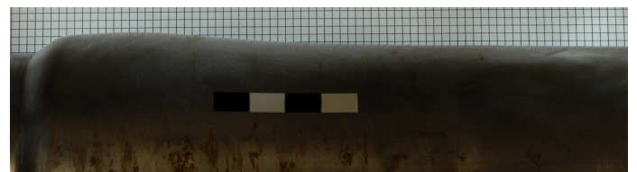
FIGURE 10. TUBE 7 AFTER 3 DETONATIONS OF INITIAL PRESSURE P_0 = 3 bar. THE GRID SPACING IS 5 mm.
