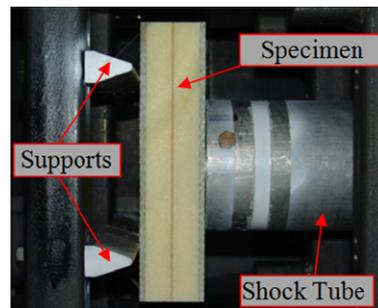
Fig. 10. (Left) Schematic of muzzle section showing transducers. (Right) Image of specimen and shock tube.
