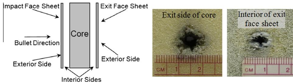
Fig. 12. (Left) Sectioning of specimen for post mortem damage study (Right) High velocity damage on interior of specimen.
