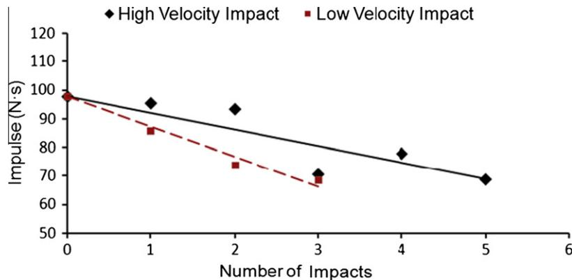
Fig. 26. Impulse generated from blast loading pressure data.
