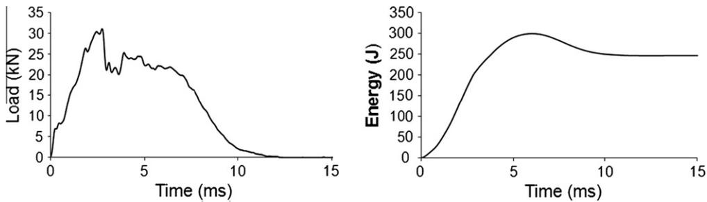
Fig. 16. Typical low velocity impact load and corresponding energy.
