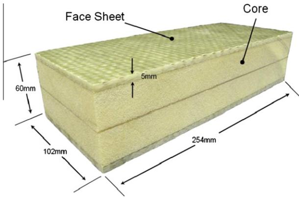
Fig. 2. Image of sandwich composite specimen and dimensions.
