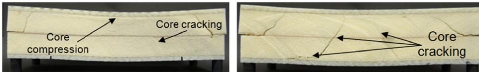
Fig. 19. Post blast images of core.
