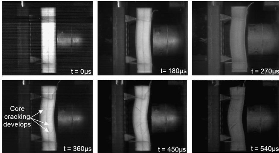
Fig. 17. Blast loading of an undamaged specimen.
