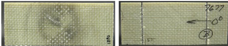
Fig. 18. Post blast image of impact face sheet and back face sheet.
