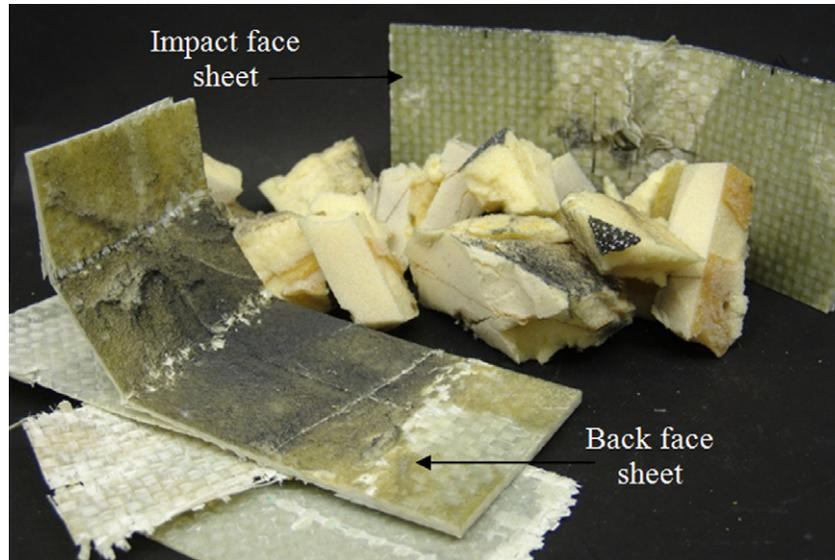
Fig. 23. Post blast image of a specimen that had been subjected to three low velocity impacts and a subsequent blast loading.
