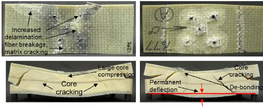
Fig. 21. Post blast image of a specimen with a high level of high velocity impact damage.
