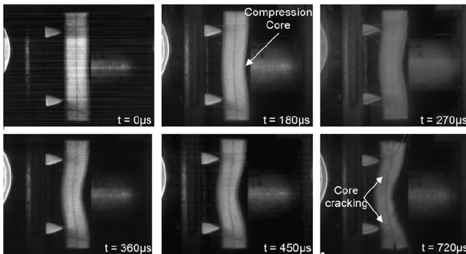
Fig. 20. Blast loading of a specimen with a high level of high velocity impact damage. Energy absorbed during impact experiments = 2108 J.
