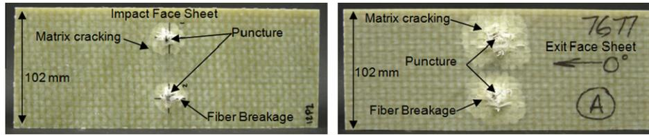
Fig. 11. (Left) Typical impact face sheet damage from high velocity impact (Right) Typical exit face sheet damage.
