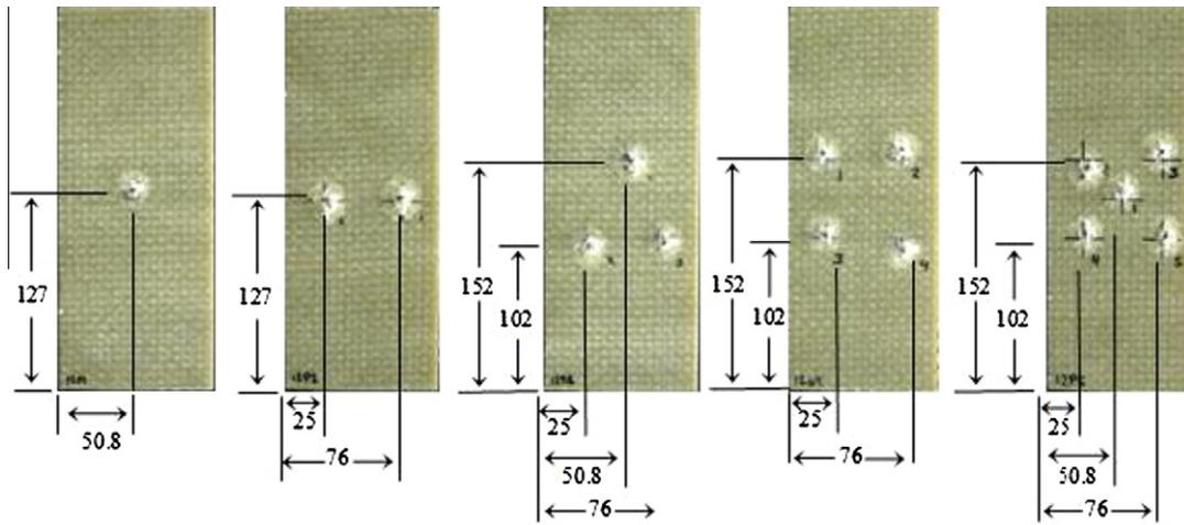
Fig. 4. Impact locations for high velocity impacts (dimensions in mm).
