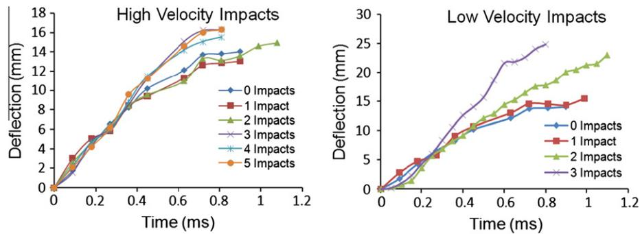
Fig. 24. Deflection of back face sheet during blast loading of specimens with high velocity impact damage (left) and low velocity impact damage (right).
