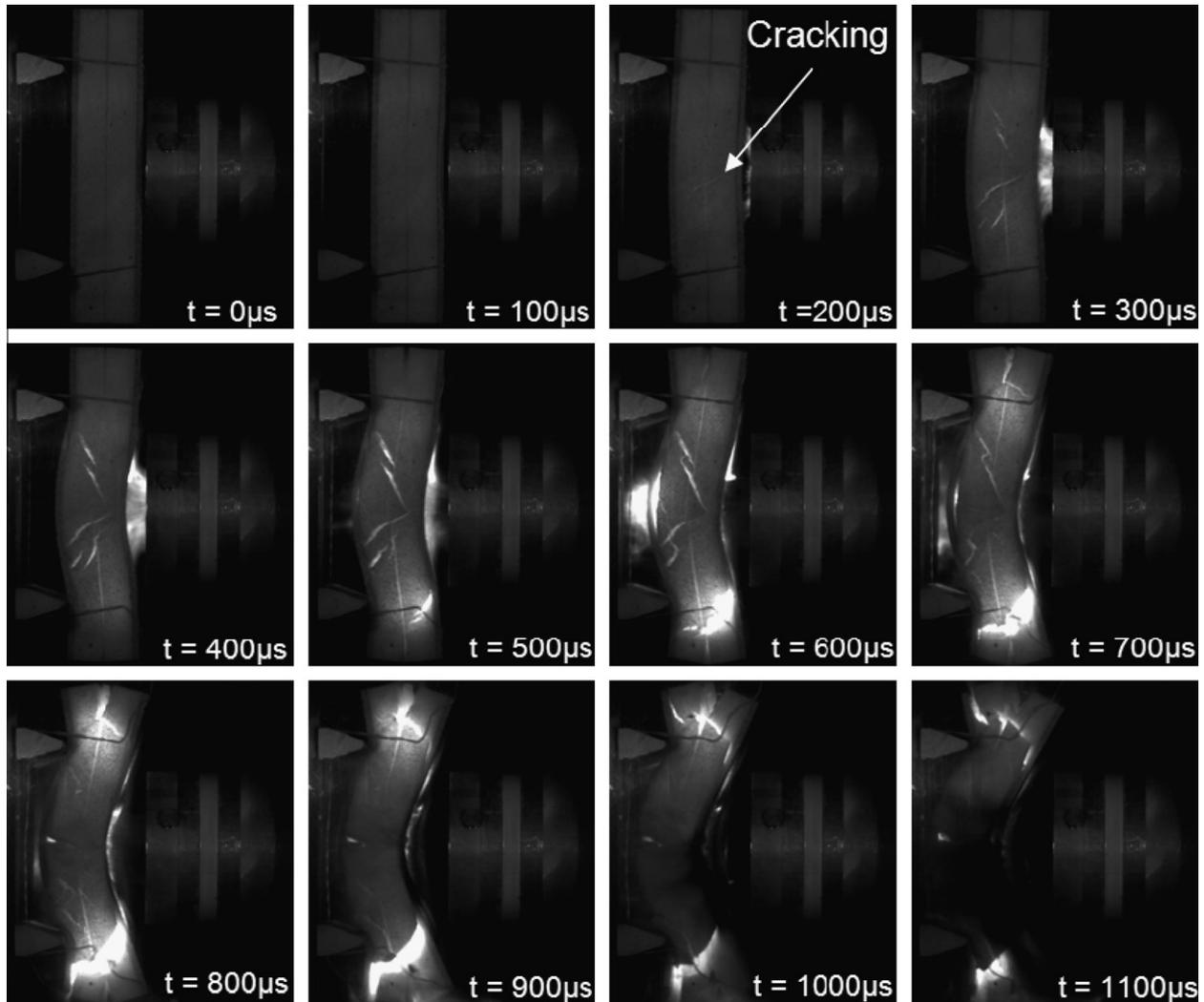
Fig. 22. Blast loading of a specimen with damage from three low velocity impacts.
