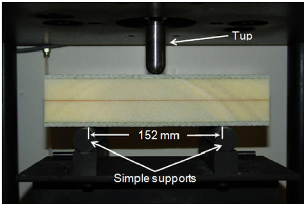
Fig. 7. Specimen placed in simply supported condition for low velocity impact.
