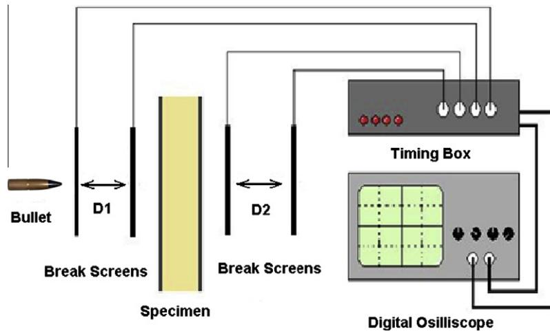
Fig. 3. Schematic of the experimental set up for high velocity impacts.
