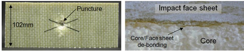
Fig. 14. Typical low velocity impact damage. (Left) Face sheet. (Right) Core/face sheet de-bonding.
