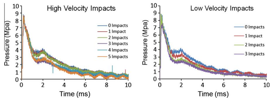
Fig. 25. Pressure time history of blast loading specimens with high velocity impact damage (left), and low velocity impact damage (right).
