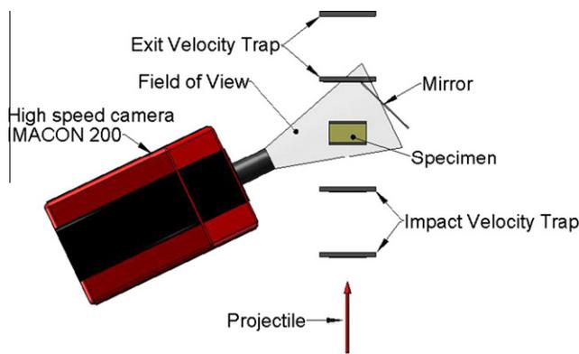
Fig. 5. Top view of high velocity impact experiment set up with Imacon 200 high speed camera.
