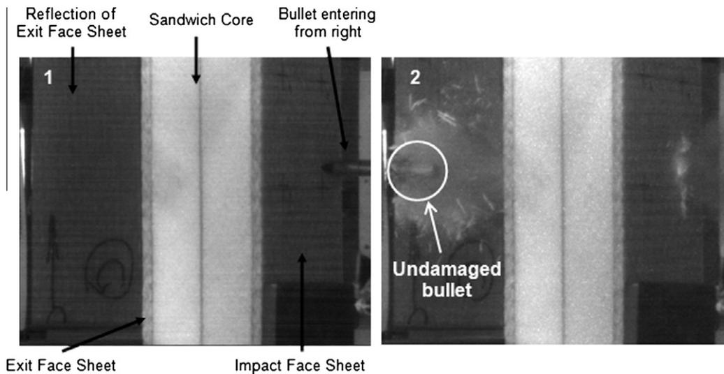
Fig. 6. High speed images of bullet impact showing the entry (image 1) and the undamaged bullet exiting the specimen (image 2).
