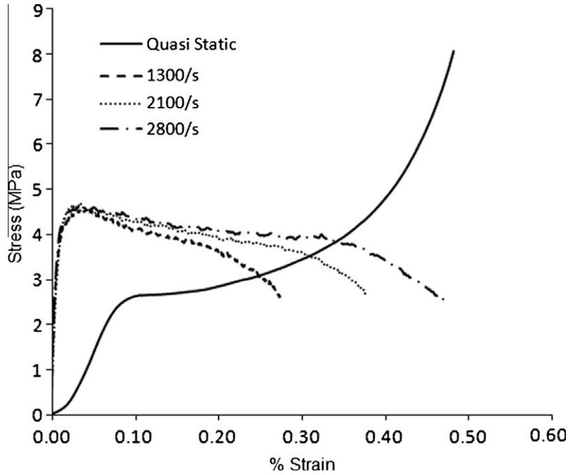
Fig. 1. Quasi-static and dynamic constitutive properties of Corecell A800.
