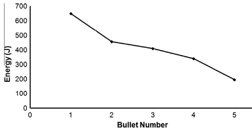
Fig. 13. Average change in kinetic energy for each high velocity impact.
