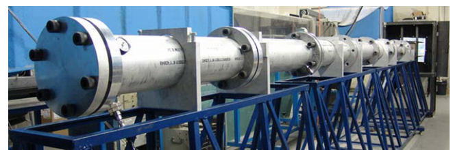
Fig. 5. The shock tube facility to produce controlled blast loading.
