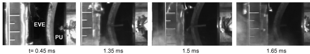
Fig. 18. Typical real-time deformation event of a polyurea/EVE layered composite plate, when subjected to blast load (0.75 MPa) EVE.
