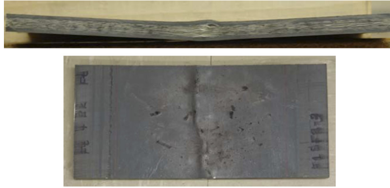
Fig. 12. Side view and strike face view of PU/EVE/PU layered sandwich plates after being subjected to shock blast loading of input pressure 1.17 MPa.
