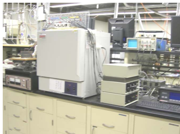
Fig 2. Entire kinetic IMS apparatus to measure rates of decomposition of explosives.
