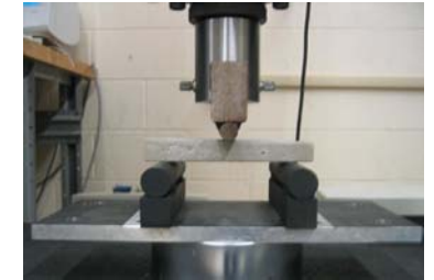
Fig 4. Instron instrument measured flexural strength (ASTM C348-97).
