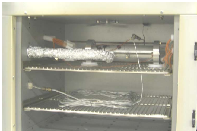
Fig 1. Kinetic ion mobility spectrometer inside oven so all components within 1C.
