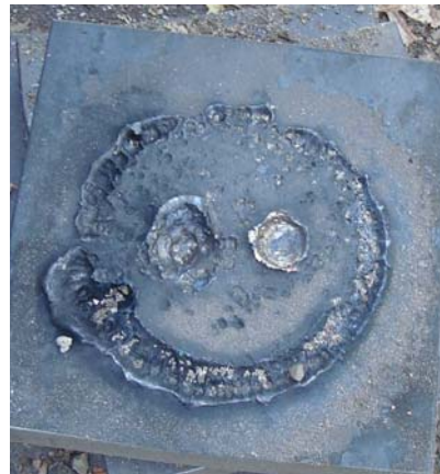
Far Left: Fig 12: Witness plates illustrating more powerful NM/DETA mix (test series 2); All plates have TM-C (48/48/4 HP/H 2 O/EtOH) as acceptor mix, top plates are Shots #5 & #15 with NM/DETA outer & bottom plates are Shots #3 and #14 with TM-A (60/27/13 HP/H 2 O/EtOH). Left: Shot #3 from Test Series 3 illustrating two dents.
