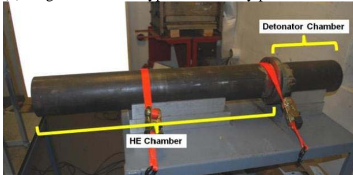
Fig 2: Explosively driven shock tube (1)
