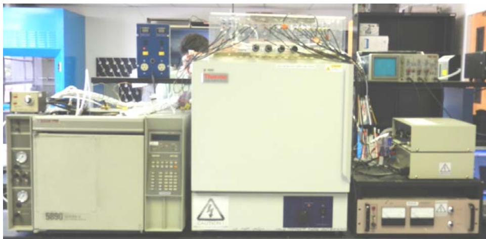
Fig. 5. The combination of gas chromatograph with kinetic IMS (inside oven) to obtain rate data free of impurities of sample. This work was started late in summer 2011 and is now in-progress.
