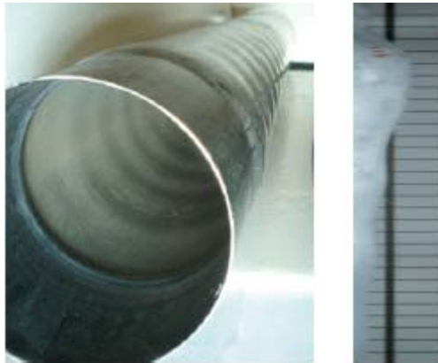
Figure 2. Stainless steel specimen tube subjected to five repeated detonations of mixture \text{C}_2\text{H}_4\text{--O}_2 and initial pressure 2 bar. The picture on the right is placed on a 5 mm grid and stretched horizontally to emphasize the periodic deformation mode.
