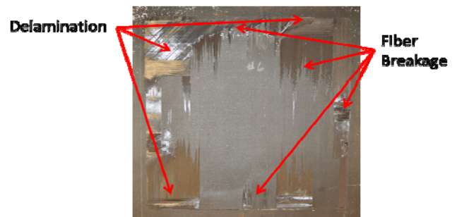
Figure 10: Post-mortem image of flat panel
