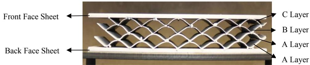
**Fig. 20** Sinusoidal graded sandwich specimen with white paint - AABC Core
