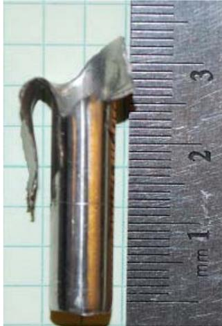
FIG. 9. Recovered thin-walled confiner after detonation of a non-ideal explosive fails.
