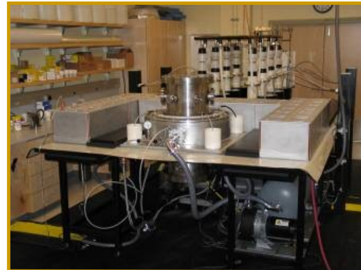
Compact Pulse Power Machine at WSU, to be used in our impact experiments
