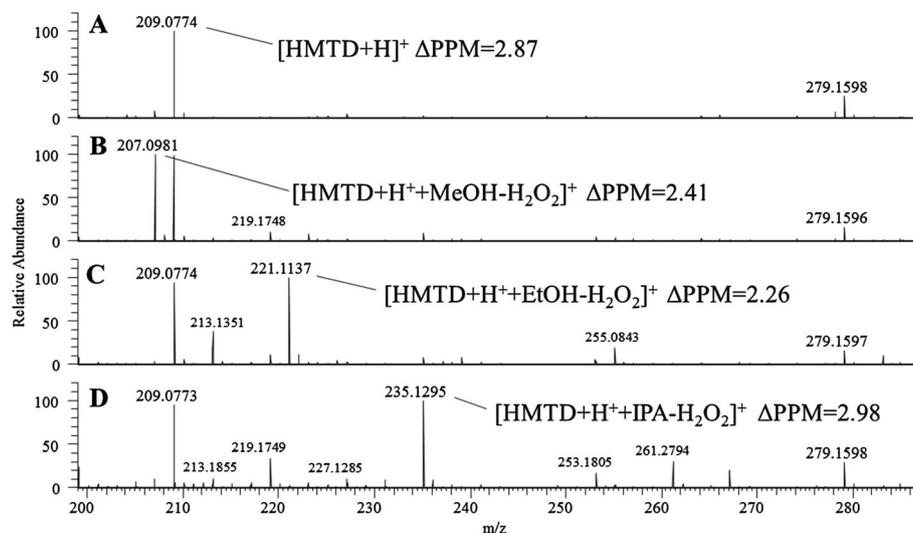
**Figure 3.** Infusion of HMTD standard solutions (5  $\mu\text{g}/\text{mL}$ , 50:50 v/v) in (A) acetonitrile/water, (B) methanol/water, (C) ethanol/water, and (D) isopropanol/water.
