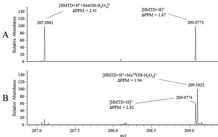
**Figure 4.** Infusion of HMTD standard solutions (5  $\mu\text{g}/\text{mL}$ , 50:50 v/v) in (A) methanol/water and (B)  $[^{18}O]$ -methanol/water. Circled areas are expanded insets within each spectrum.
