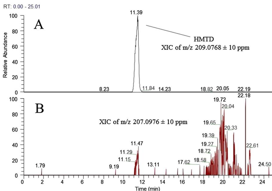
**Figure 6.** HPLC analysis of HMTD stored in methanol/water (50:50 v/v) under ambient conditions for 5 days. Extracted ion chromatograms (XICs) for (A) HMTD ( $\sim 3 \times 10^6$  height counts) and (B) the methanol adduct ( $m/z$  207.0976,  $\sim 4 \times 10^3$  height counts).
