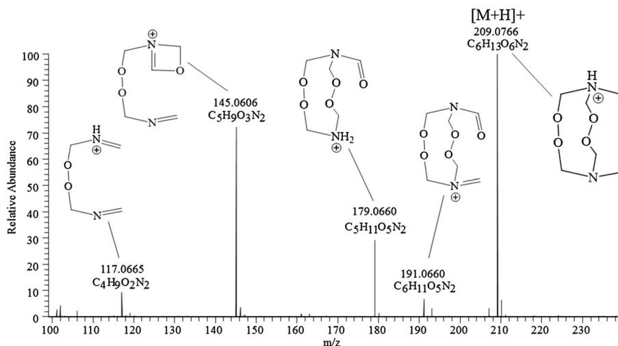
**Figure 1.** HMTD and tentatively identified fragment ions produced in the source using APCI<sup>+</sup>, with acetonitrile/water with 0.1% acetic acid mobile phase.
