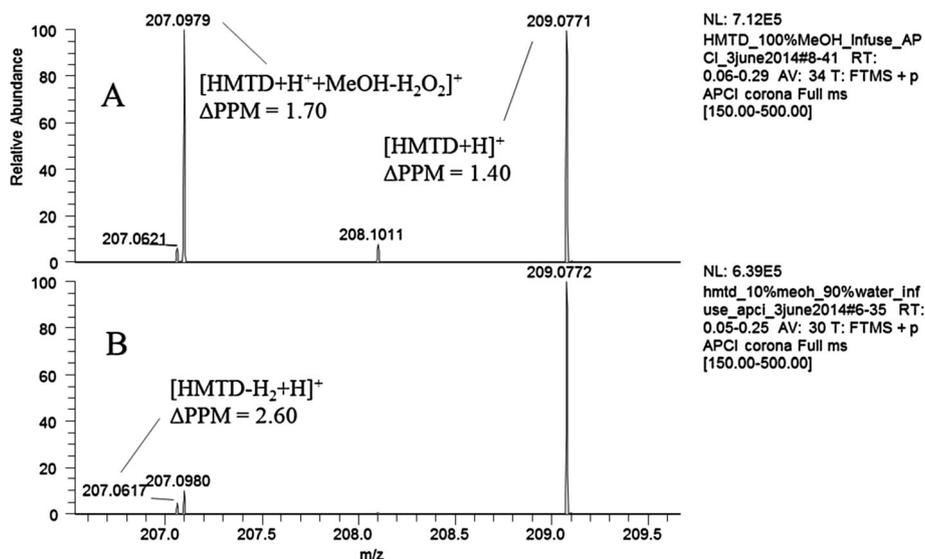
**Figure 2.** Infusion of HMTD standard solutions (5  $\mu\text{g}/\text{mL}$ ) in (A) 100% methanol and (B) 10% methanol/90% water. Note that, with the 10% methanol solution, the peak associated with  $[HMTD-H_2+H]^+$  is ~50% of the  $[HMTD+H+MeOH-H_2O_2]^+$  peak, but only 5% relative abundance in both spectra.
