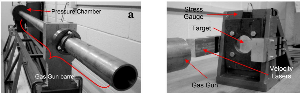
Figure 2. Photograph of a.) the experimental light gas gun and b.) the target and fixed back holder
