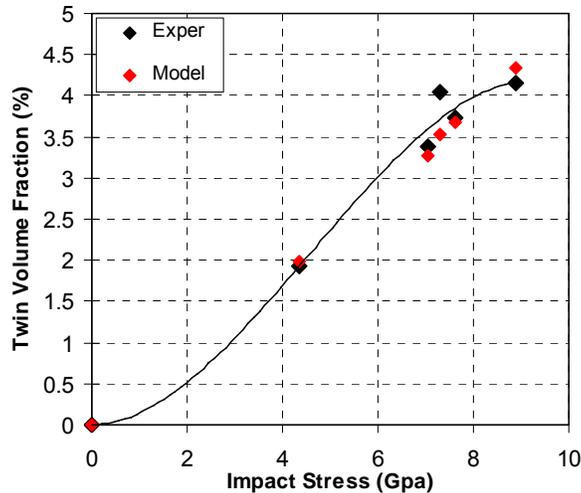
Figure 8. Comparison of experimentally measured and analytically computed twin volume fraction as a function of impact stress.
