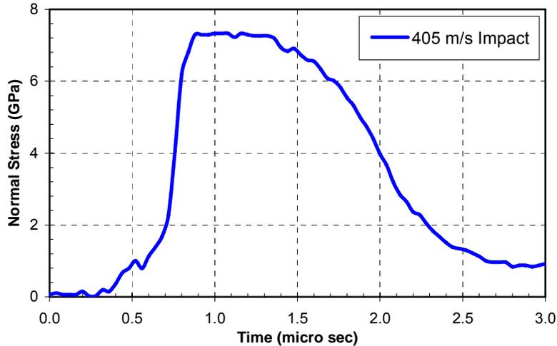
Figure 3. Impact Stress recorded with manganin gauge at the back surface of target disk during a 405 m/s impact
