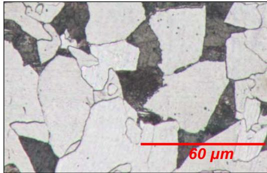
Figure 1. Micrograph of as received A572 grade 50 structural steel.
