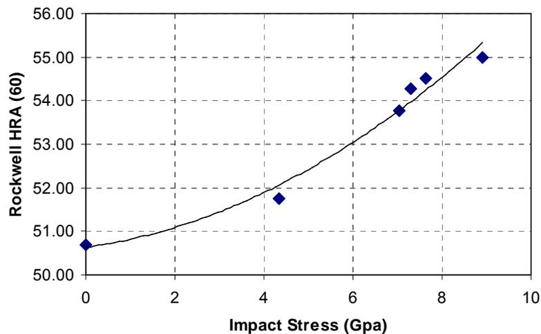
Figure 6. Post-impact macro hardness as a function of impact stress
