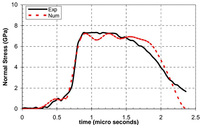
Figure 7. Experimental and numerical stress history at the back of the target specimen.
