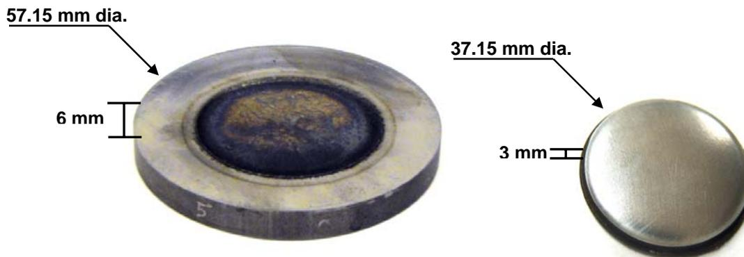
Figure 4. Impacted steel target specimen and deformed projectile
