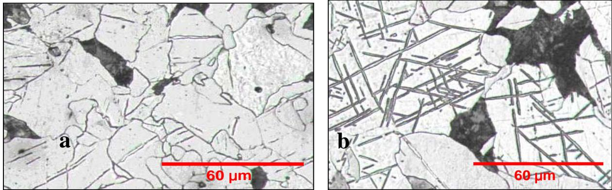
Figure 5. Example of optical micrographs of post impact steel specimens a.) 7 GPa peak stress yielding 3.4% twins, b.) 9 GPa peak stress yielding 4.3% twins.
