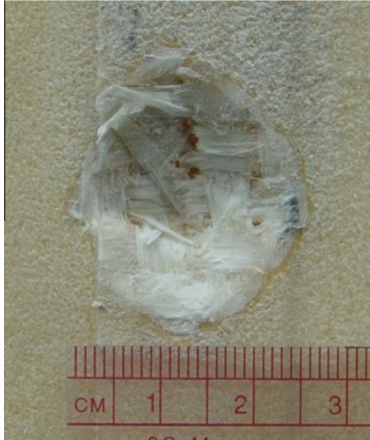
Fig. 15. Core damage due to low velocity impact.
