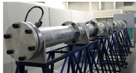
Fig. 9. Diagram and image of shock tube.
