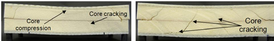
Fig. 19. Post blast images of core.
