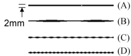
**Fig. 9** (A) Straight 2 mm thick water-sheet, (B) water sheet with a wavelength of 50 mm, (C) water sheet with a wavelength of 8.3 mm, and (D) water sheet with a wavelength of 4.2 mm. *NOTE: All the water sheets with perturbations are between 0.3 cm and 0.1 cm thick.*
